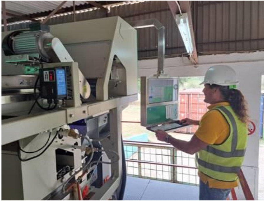
Figure 2. Optical sorter, extracting emeralds and emerald bearing material from the ore
