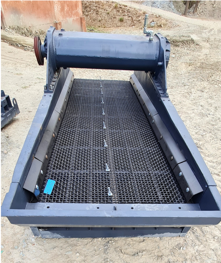
Figure 3. New Double Deck Sizing and washing Screen to replace the Trommel screen.
