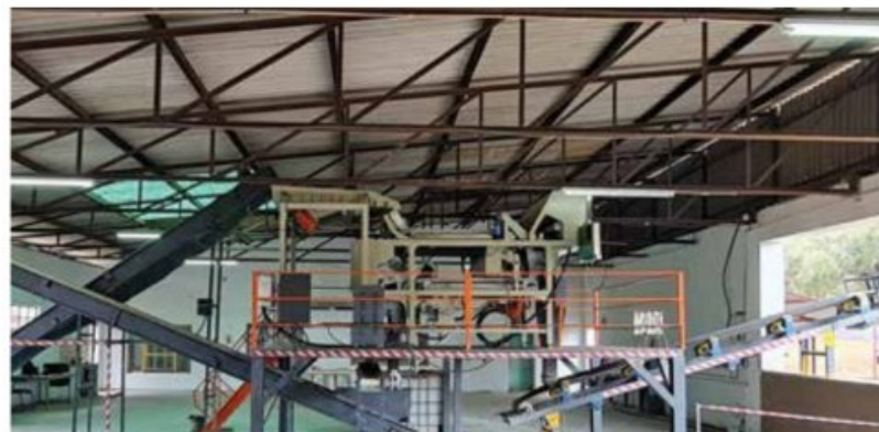
↑ The Angelon optical sorter at Gravelotte eliminates the need for hand sorting
